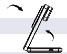
Spin out from right to left, rotate to adjust by 90° or 180° (for charging the watch).
